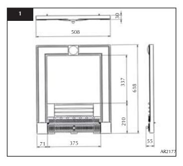
Diagram 2 shows the Winchester Front dimensions for the E-Box, E-Studio Conventional and Balanced Flue:
